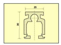
Material: AIMgSi 0.5 Heat treated anodized aluminum
