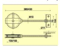
Nominal diameter of wheel: 100 and 150 mm Max. setting: 200 mm
