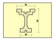
Material: AlMgSi 0.5 Heat treated anodized aluminum
